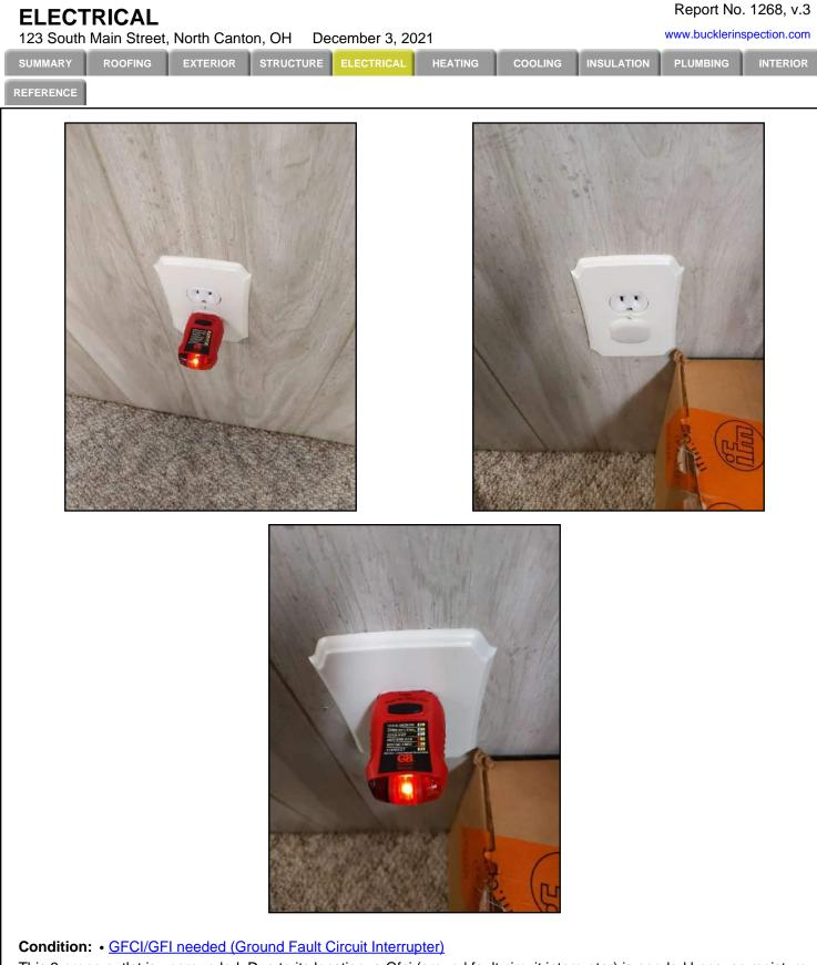
This 3-prong outlet is ungrounded. Due to its location, a Gfci (ground fault circuit interrupter) is needed because moisture can create an electrical hazard. The Gfci should be labeled as no ground for safety. **Implication(s)**: Electric shock
